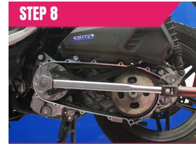
Tighten the variator with torque wrench with the manufacturer's torque
