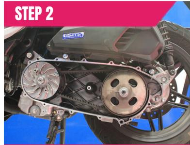
Remove the cover of the automatic transmission system
