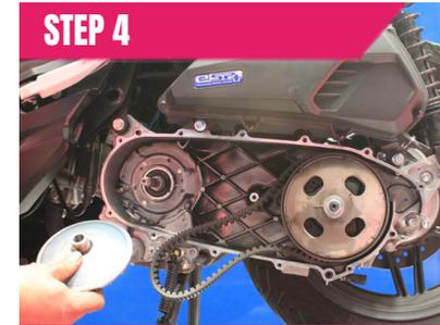
Remove the original drive and any grease, oil or dust residues.
