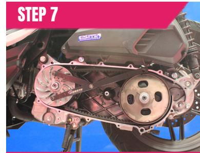
Install the semi-pulley and lock the the variator
