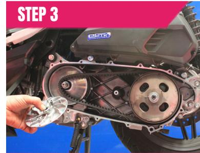
Remove the drive half-pulley from the variator to release the belt
