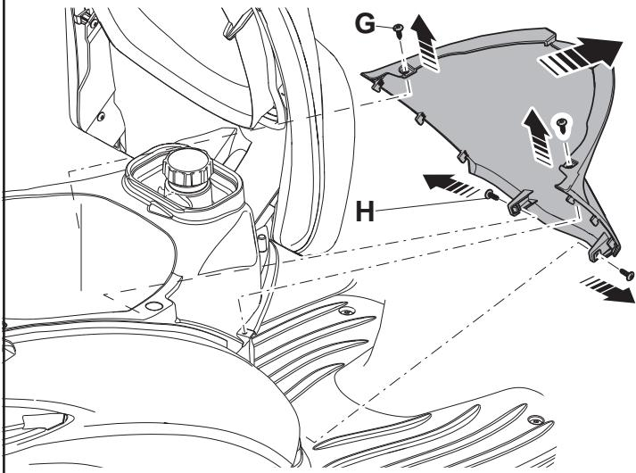
**G** Undo the two top fastening screws **G** and the two bottom ones **H** of the spark plug inspection hatch. Close the saddle and remove the hatch from the scooter.
