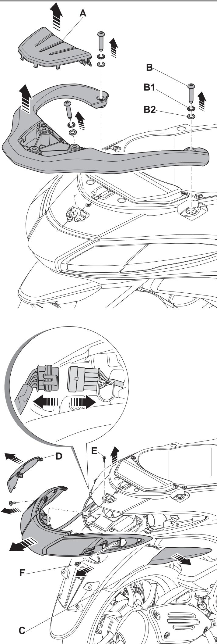
Remove the plastic cover of the luggage carrier **A** by lifting gently, from bottom to top with a screwdriver.
