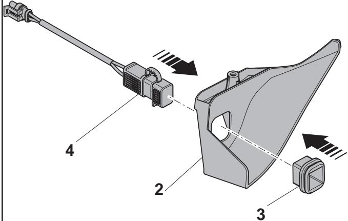
**G** In the right bag **2**, provided in the kit, insert the rubber gasket **3** of the USB port **4** housing from the outside towards the inside.
