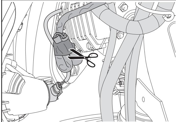
Cut the belt fixing the connector **AD** to the wiring harness of the left turn indicator.
