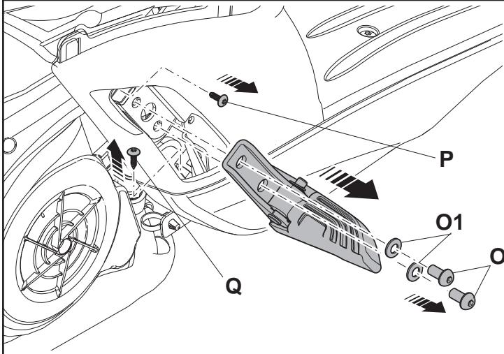
**GB** To remove the left passenger footrest undo and remove the two fastening screws **O** with their washers **O1**.
