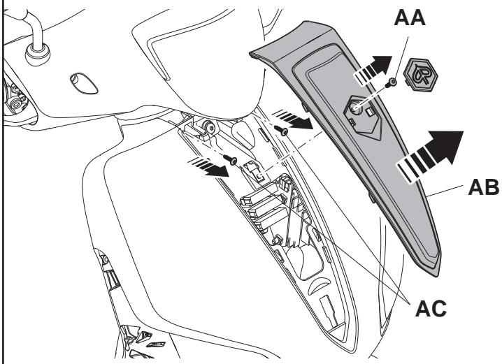
**G** Remove the plaque with the "PIAGGIO" logo, then undo the screw **AA**.
