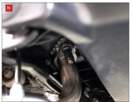
N) Adjust the system so that it sits nicely, is clear of moving parts and is under no stress. Then starting with the header nuts, then the clamp and finally the 2 silencer mounting bolts fully tighten everything.
