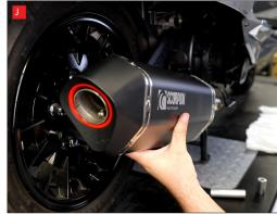
I) Place the silencer face down on a cloth to avoid damaging it and then install the silencer bracket with the supplied hardware following the line diagram on the 1st page. Fully tighten the mounting bolts.
