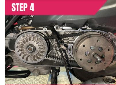
Remove the clutch nut, clutch washers and transmission cover.
