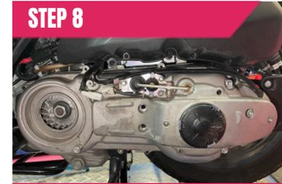
Reinstall the transmission cover, tighten the clutch nut to the original torque (7.5KG/75NM) and replace all bolts.
