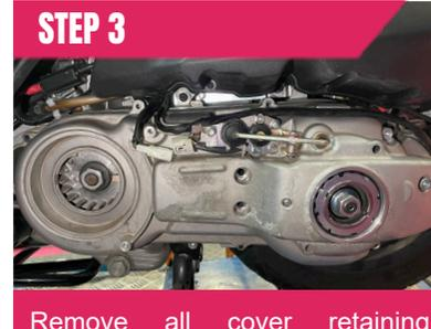
Remove all cover retaining screws, the plastic cover and disconnect the terminal block.
