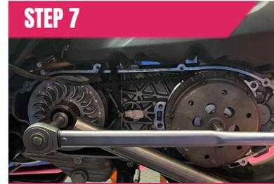
Install the semi-pulley, lock the variator and tighten the variator with a torque wrench.
