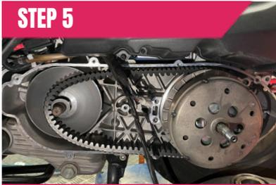
Uninstall the semi-pulley and remove the standard variator and all grease, oil or dust residues.
